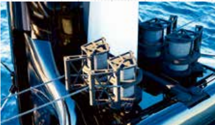
Left: heel and deck bearings for a modern rig. Above and right: four captive winches on each truss. The sail handling equipment is now all mounted on a common chassis unit on each truss
